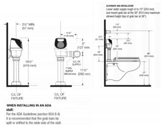
Per the AUA Guidelines (section 004.9.4) it is recommended that the grab bars be split or shifted to the wide side of the stall. If grab bars must be present over the valve, use the alternate ADA installation as shown to the right.
